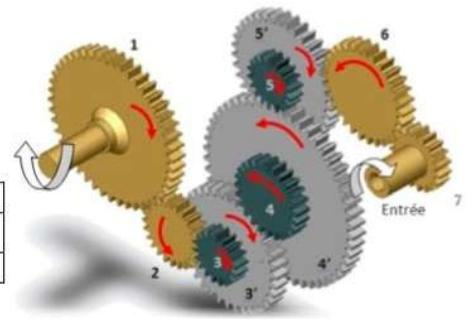
$$\text{Relation de Willis : } k = \frac{\omega_{s/0}}{\omega_{e/0}} = (-1)^6 \frac{\prod Z_{\text{menantes}}}{\prod Z_{\text{menées}}} = \frac{30 \times 42 \times 26 \times 38 \times 24 \times 32}{42 \times 54 \times 82 \times 48 \times 32 \times 65} = 0,05$$
