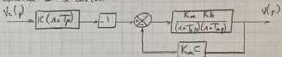
Donc :  $H_1(p) = \frac{V(p)}{F_{\text{rel}}(p)} = K(1+T_p) \frac{\frac{K_m K_b}{(1+T_p)(1+T_m)}}{1 + \frac{K_m K_b K_c}{(1+T_p)(1+T_m)}}$
